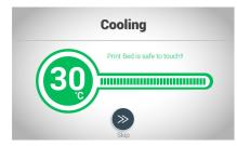
After the printing, the screen will show the temperature of the print bed. Take out the printed object after the temperature of the print bed is cooling down to the room temperature.
