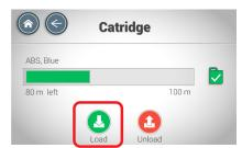
4 Select "Filament" > "Cartridge " > "Load".
