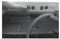
If the filament is stuck at the entrance of the guide tube, please press the release arm by the entrance to extract the stuck filament.
