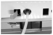
After removing the filament, plug the filament tube directly back to its original position to complete the re-installation.
