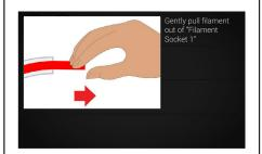
Filament is unloaded from extruder automatically. Gently pull filament out from the guide hole when prompted.
