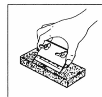
The illustration shows a close-up of a hand holding a honing guide. The guide is a rectangular block with a slot for a blade. A blade is partially inserted into the slot, and the hand is shown applying pressure to the blade as it rests on a textured, rectangular sharpening stone.
